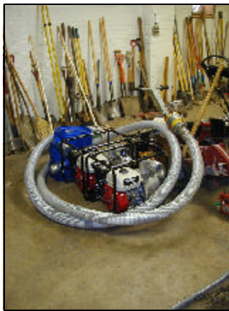
These trash pumps, which are designed to retrieve water, mud and debris, were rented to be used to clean the aftermath of Hurricane Frances.
